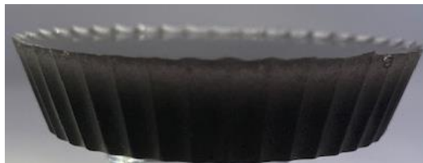
Figure 4 – Filled polymer with a visible filler gradient (low conc. on top, high conc. on bottom).
